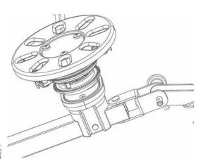
Line Power Pad up with the PCB mount on the Power Rail.Then push down firmly until clamp snaps in place.
