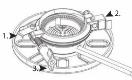
Unlatch nut (1) and clamp (2) locking tabs. Then unscrew wingnut (3).
